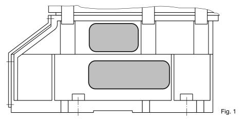
The identity code and serial number are given in addition to the standard technical specifications. These two numbers must always be quoted when making any enquiries as they enable distinct identification of the type of metering pump.
